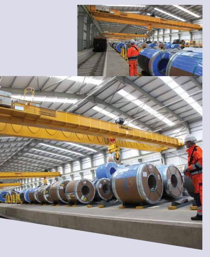
Each double box-beam girder crane spans an exceptional 35m. Due to the high frequency of movements, Street VX hoists were also supplied. These were custom designed and built for the application enabling them to be used at the highest duty rating of M8.
