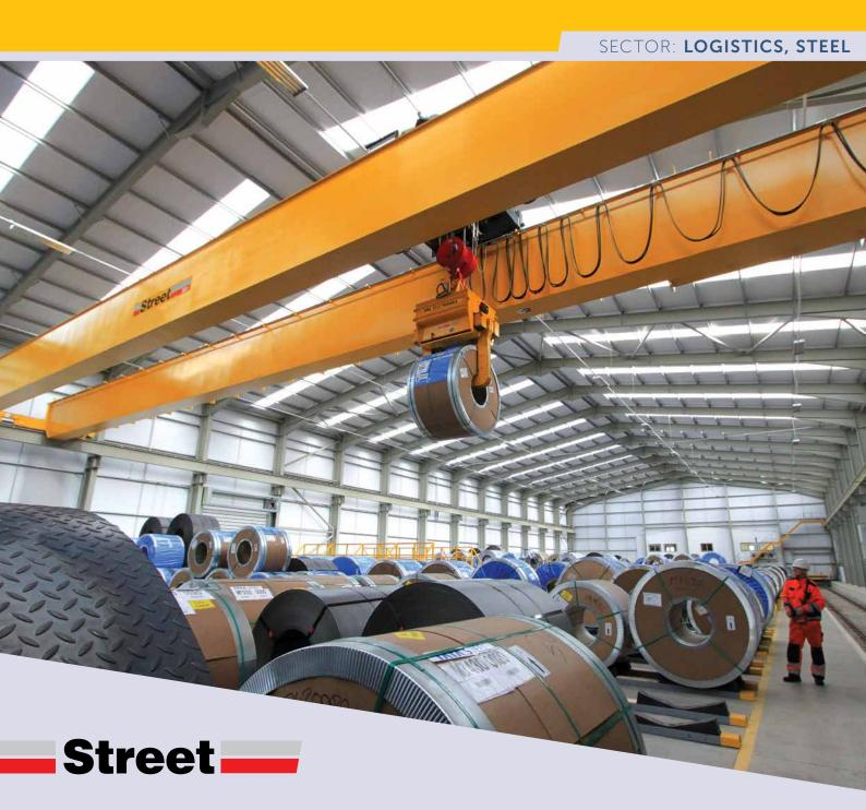
Street's 30-tonne overhead cranes are playing a crucial role at this high-capacity steel warehouse.
